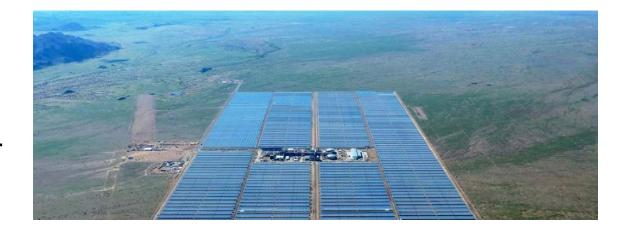
Above is a photo of the 50MW Khi and 100 MW Kaxu solar project where they combined concentrated solar power technology with saturated steam and molten salt energy storage.
